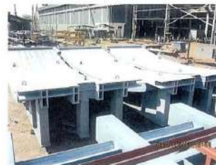
Settler Flash Furnace: Bottom Saddle (109.380 kg)
