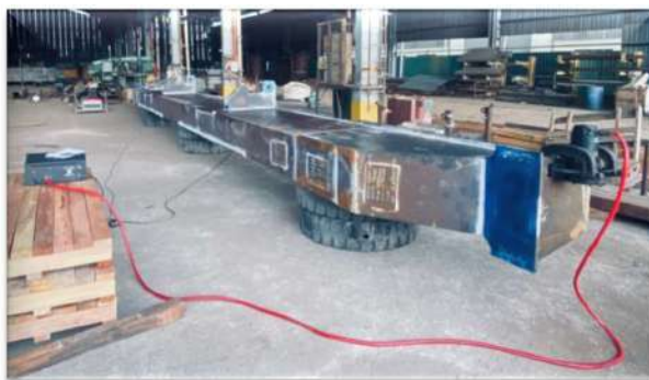
VIBRATORS STRESS RELIEF MACHINE (HB300+K5) – 100 TONS
