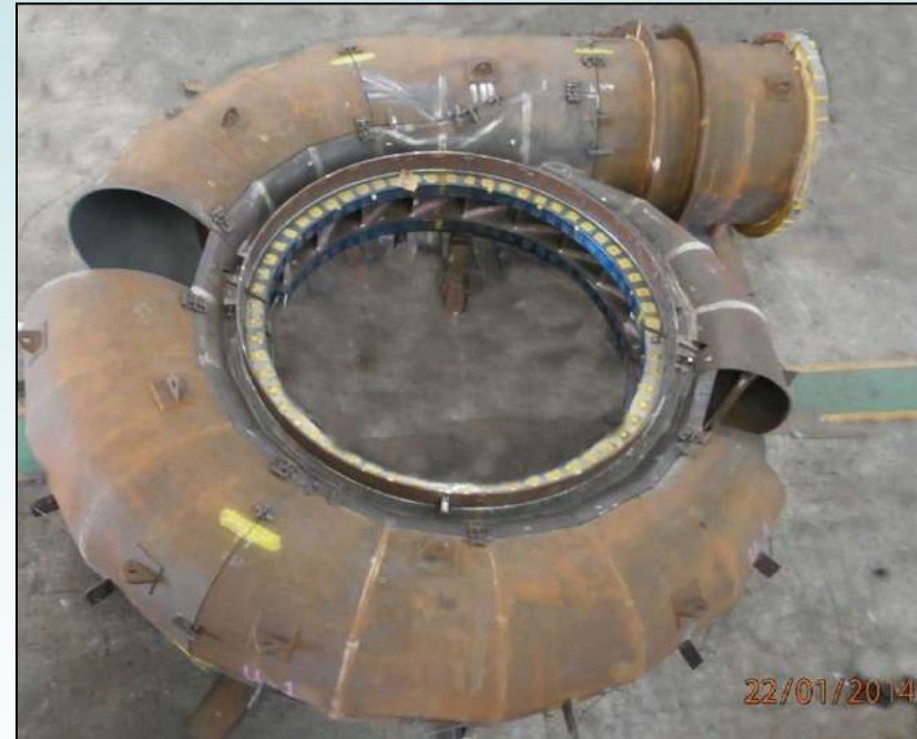
Spiral Case and Stay Ring Unit#1 - Completed on Feb 2014
