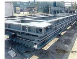
Settler Flash Furnace: Grillage Beam (26.800 kg)
