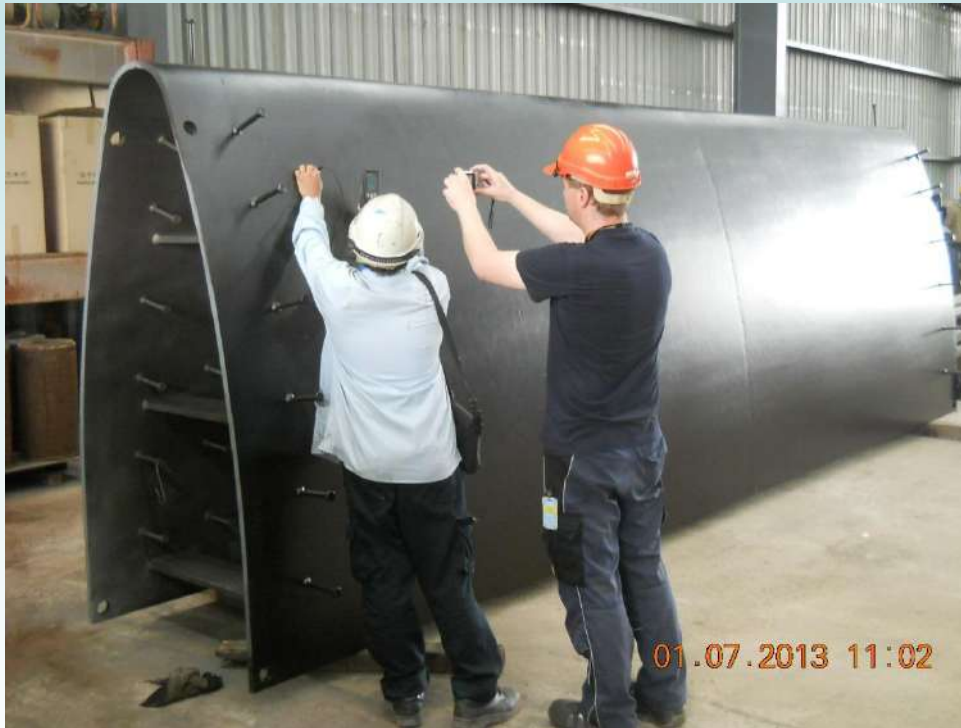
Pier Nose Liner -Completed & Delivery October 2013
