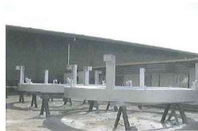
Koniambo Furnace Water-cooled Roof Dome Skew Ring Total Mass: 4600 Kg
