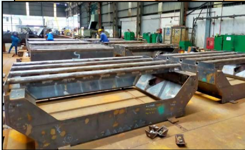
Fabrication of Grate Casing Tube
