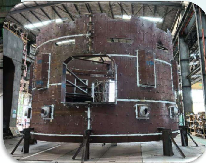
Pier Nose Liner
