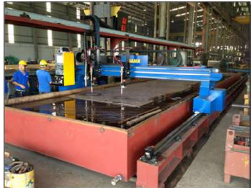
DAMA - HIGH DEFINITION PLASMA CNC FLAME / CUTTING MACHINE
