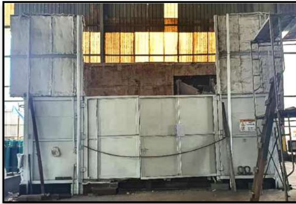
PWHT FURNACE (GAS FIRING) SHAH ALAM (BLOCK C FRONT) 6mW x 6mL x 4mH
